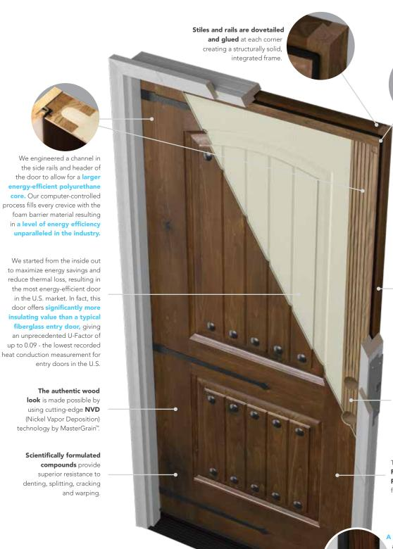
To enhance efficiency and accommodate more insulation, we thickened the door and sidelites from the standard 1¾" to 2½" which is 43% thicker than standard exterior doors. We also engineered a dual-perimeter seal for the entry door to create a superior barrier against drafts and energy leaks.
